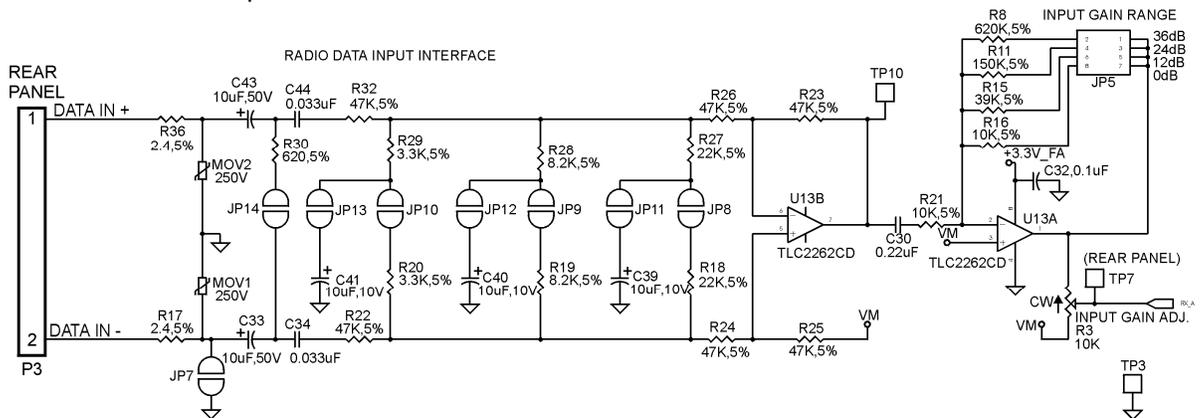
The input is capacitively coupled for DC blocking and is MOV protected. When interfacing to a radio, connection should be discriminator audio, before deemphasis (flat audio). Data input + should be jumpered for high impedance and data input - should be jumpered to ground.
