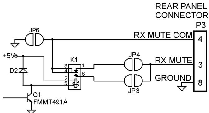
When using the mute feature, it is especially important to attach station ground to the back barrier strip of the C Plus at P3 pin 8 or P2 pin 10. Audio common used at the *Data In -*, even if it is ground, is not sufficient.
