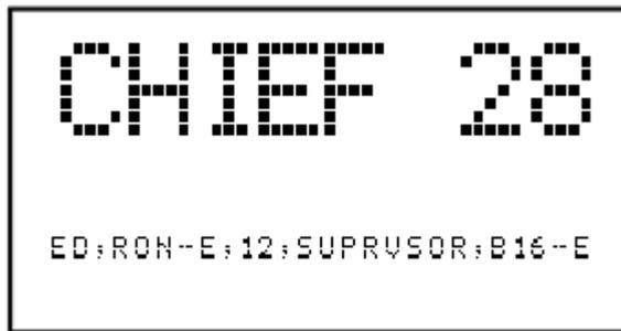
In this example, the C Plus also has the optional feature "Alias" installed. Note the secondary display. The ANI received just before "CHIEF 28" was from unit B16 and the message type was "E" (Emergency). The ANI received before B16 came from SUPRVSOR and the message type was a normal PTT ANI. The one before that was a PTT ANI from unit 12. If the Alias feature was not installed, all ANI would be numerical only.
